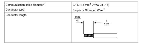
\*1 When inserting two wires into one terminal connector, the simple wire diameter is 0.08 to  $0.5 \text{ mm}^2$  (AWG 28 to 22), and the stranded wire diameter is 0.08 to 0.75 mm<sup>2</sup> (AWG 28 to 20).
