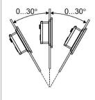
When installing this product in a slanted position with an incline more than 30°, the ambient temperature must not exceed 40 °C (104 °F). You may need to use forced air cooling (fan, A/C) to ensure the ambient operating temperature is 40 °C or less (104 °F or less).
